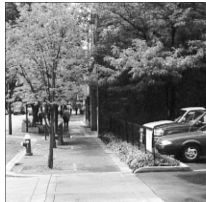
Where a parking lot abuts a public sidewalk, provide a landscape buffer. This one includes ground covers and a fence.
