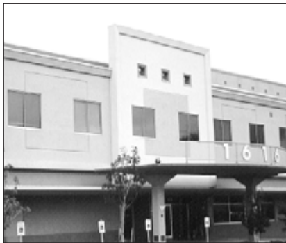
Stucco that is detailed to convey a sense of scale and provide visual interest is an appropriate material treatment.
