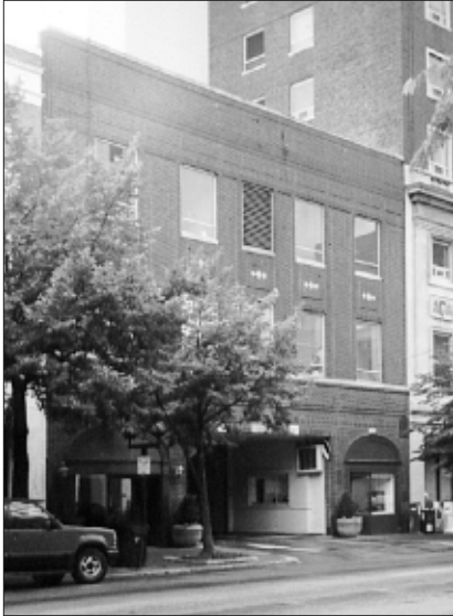
Narrow curb cuts, such as this, can provide access to internal parking facilities while minimizing crossing conflicts with pedestrians.
