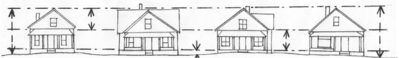
Illustration 17: New construction should be consistent with existing foundation and floor-to-ceiling heights.
