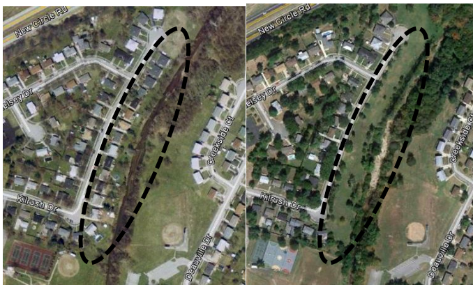
Aerial photographs Kilrush Drive nearby Wolf Run from 2002 (left) and 2010 (right). Eighteen residences in the area that were constructed in the floodplain in the 1960s were purchased and demolished as part of LFUCG's Stormwater Capital Improvement Projects.
