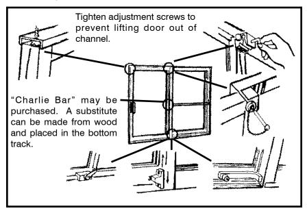
Numerous locking devices are available for sliding windows and doors. Those operated by keys are recommended for better security.
