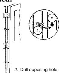
2. Drill opposing hole in door jam to receive the protruding screw or nail. When the door is closed, the hinge pin may be removed, but the door will be held firmly in place.
