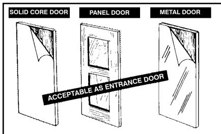
Solid Core, Panel Doors, and Metal Doors offer good protection if secured with a good lock.
