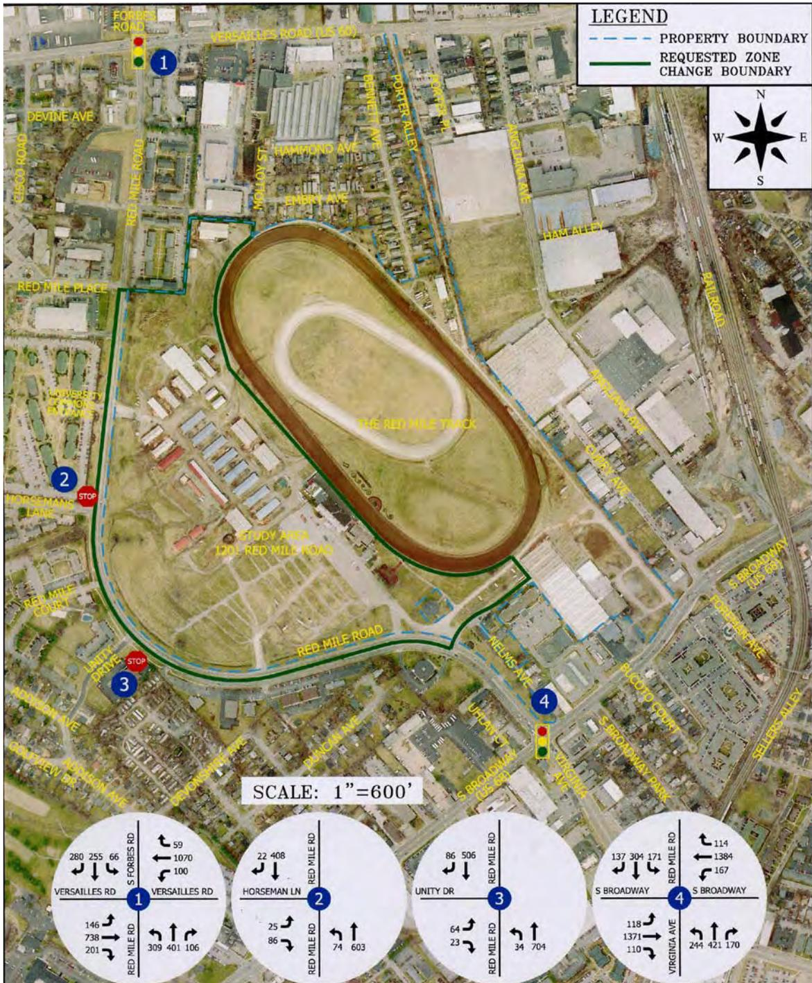
Diagram © describes traffic and turning movement counts, as well as pedestrian counts, that were collected at two signalized intersections (Versailles Road and South Broadway). It also shows counts for two un-
