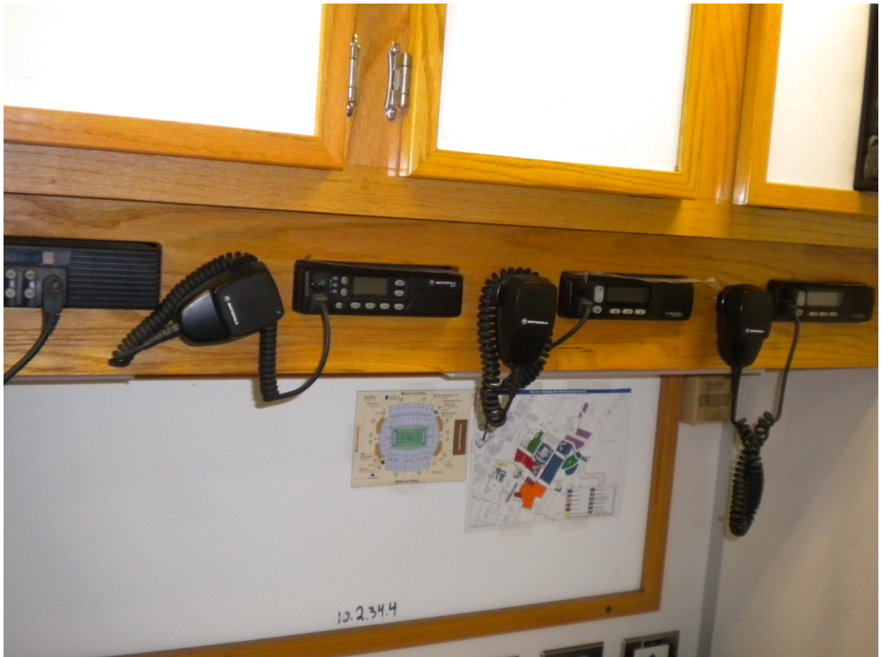
Figure 9: Some of the interoperability units installed in Division of Police's command vehicle.
